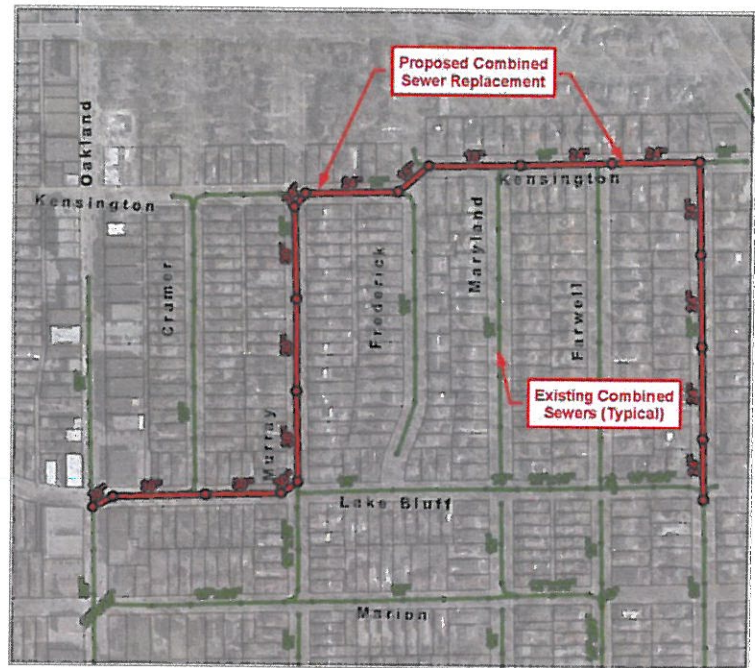
Alternate 2 Combined Sewer Upgrades
