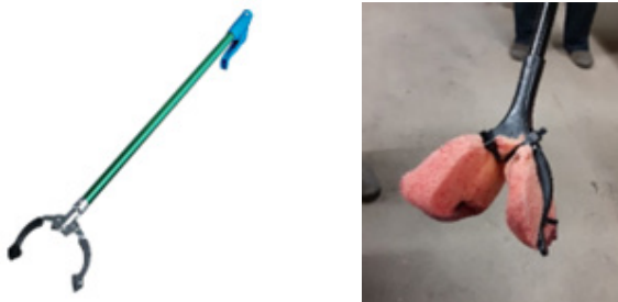
Figure 1 – Using a garbage grabber from any home improvement store (left), attach a sponge using zip ties and fasten it to the inside of the 'grabber' as shown in the photo (right).
