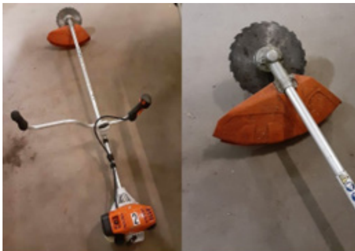
Figure 4 – (LEFT) STIHL brand forestry saw with Bike Handle mount, necessary when operating for heavy use on woody debris. (MIDDLE) Circular saw blade attached, best for woody plants. (ABOVE) The blade can be changed out to use on grasses and herbaceous vegetation. Always make sure property PPE is worn during saw work.
